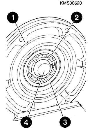
Removing cylindrical roller bearing in drive/reduction gear end shield
